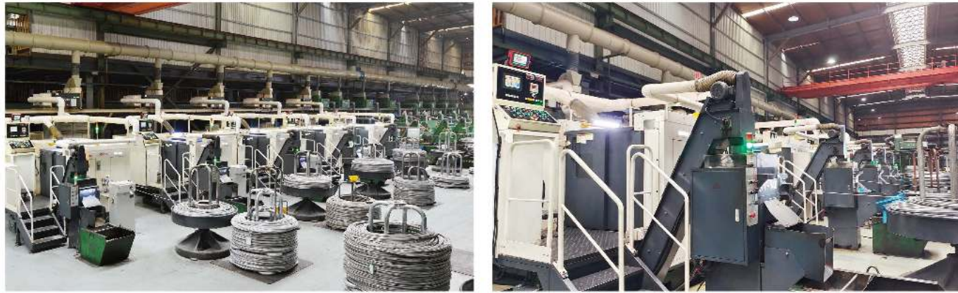
Large bolt cold forming machines up to M36 and 1-1/2"
